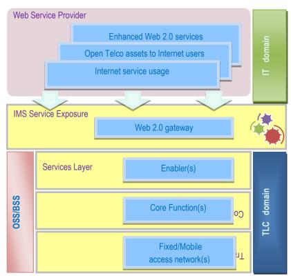
Figure 15: Platform architecture for NGN/IMS/web 2.0 service building.
