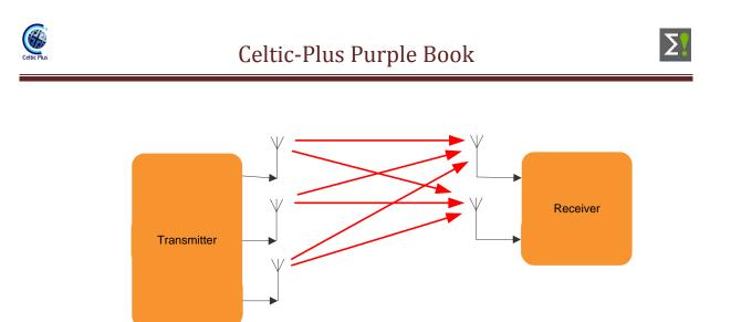
Figure 9: Multi-Antenna System Example
