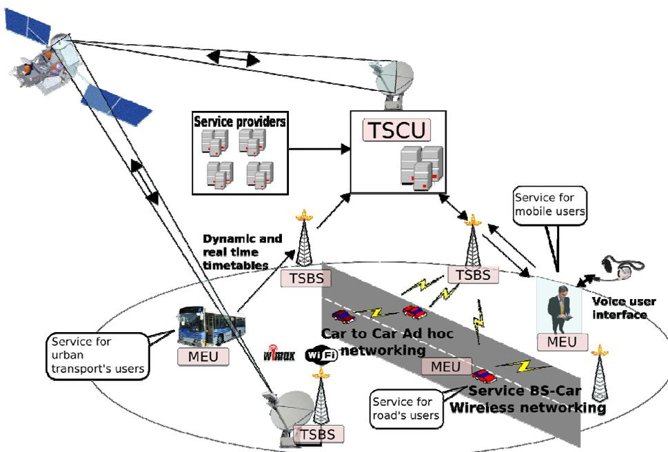
CARLINK equipment installed in test vehicles transmits position and data from sensors in real time, so it is easy to track vehicles and observe both measured and forecasted weather and traffic conditions. The platform operability, usability and necessity will be approved through few key services. These services are Local Traffic Weather Service and Traffic Management Service.
