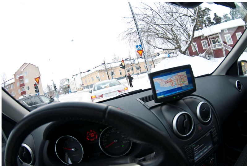
WiSafeCar pilot vehicle equipped with various sensors connected via the Sensor-unit to the Sunit on-board PC that is capable to communicate both by WLAN (IEEE 802.11p) and cellular (GPRS/3G)
