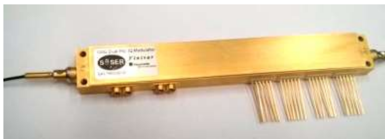
Fig. 4: Packaged 28Gbaud Dual-Pol. I/Q modulator in GaAs
