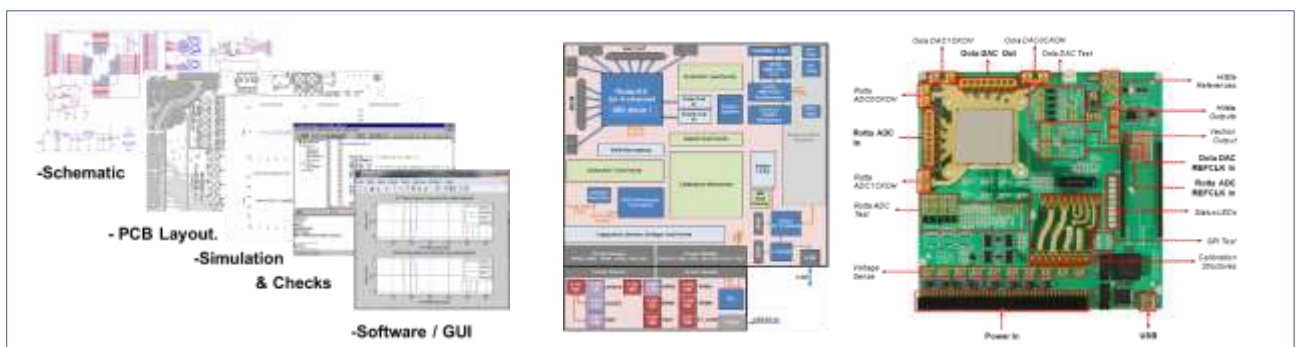
Fig. 13: Main tasks performed on the DK and basic block diagram and picture of the PCB.
