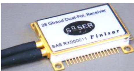
Fig. 1: Small form factor 28Gbaud dual-pol. coherent receiver (left), 56Gbaud dual pol. coherent receiver (without electrical amplifier) (right)
