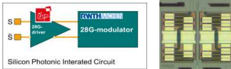
Fig. 8: Meandered modulator for 28Gbps operation co-integrated with high speed driver
