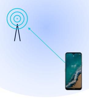
Frequency Domain Spectrum Shaping (FDSS) with spectrum extension enables up to 2 dB coverage extension
