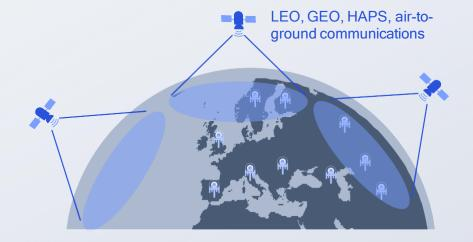
Supporting satellites backhaul communication for CPEs and direct link to handhelds (e.g., smartphones) for low data rate services
