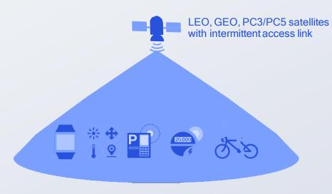
Supporting diverse use cases, including transportation, utilities (e.g., solar, oil/gas), farming, mining, environmental monitoring Utilizing sub-7 GHz band for both eMTC and NB-IoT, with LTE EPC¹ only in standalone network
