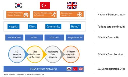
extended to accommodate the automated interactions between application-layer healthcare services and network-layered 5G services. This flexible service integration approach will provide the much-needed on-demand adaptive network quality-of-service guarantee whilst satisfying the loose coupling requirements between the applications and the network.
